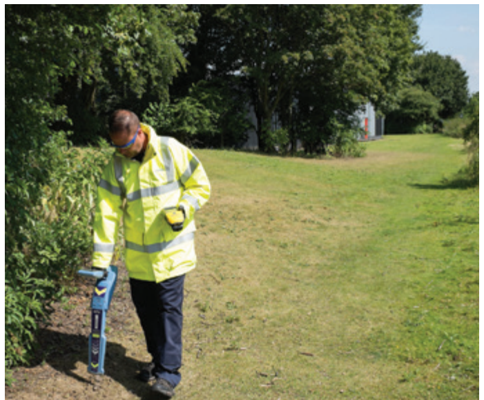
A customised solution developed for Capita that uses Bluetooth to link an underground cable locator with a hand-held GNSS and data capture software
