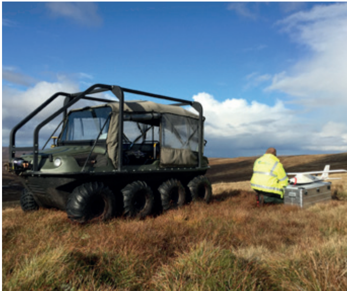
The Sirius Pro surveys to a high degree of accuracy across demanding areas, with its built-in RTK-GPS navigation system eliminating the need for GCPs
