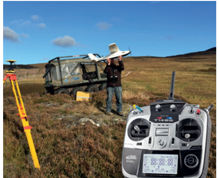
Highland Fling! Being launched by hand, there is no need for a cumbersome catapult or launch rails. The radio remote control (lower right) is used to command the platform which has a 1.6 m wingspan and a take-off weight of under 3 kg
