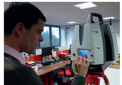
Leica ScanStation being checked in Technical Support to ensure it captures 3D data and HDR imaging at a rate of a million points per second at ranges of up to 270 m. Photo: GEOconnexion
