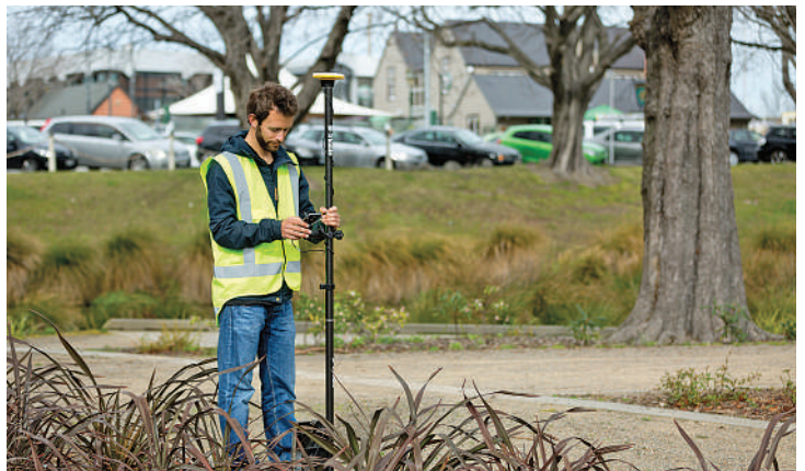
Trimble Catalyst in the field: a GNSS receiver built out of software. Photo: Trimble
