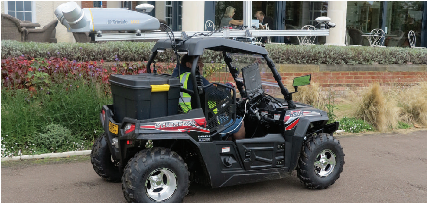
All terrain data capture using the Trimble MX2 spatial imaging system
