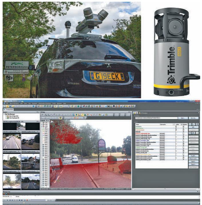
Trimble’s vehicle-mounted MX series spatial imaging systems (top left and right) combine high resolution laser scanning and precise positioning to collect geo-referenced point clouds for a wide range of requirements. Lower picture: Health and safety was a key factor in the London Borough of Merton’s use of Trimble’s MX2 mobile mapping system to acquire data relating to 380km of roads. Once captured, the data was checked and transferred into the Council’s existing asset management system.
