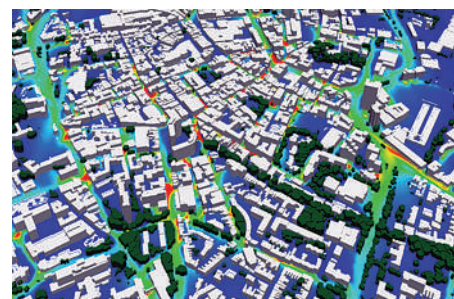
Pollution concentrations in a complex urban environment, as modelled by the FluidAir system of the University of Leicester and EarthSense Systems Ltd. This information was used to generate air quality maps for the HotSpot Mapper project within the Space for Smarter Government Programme Image © Satellite Applications Catapult Ltd
