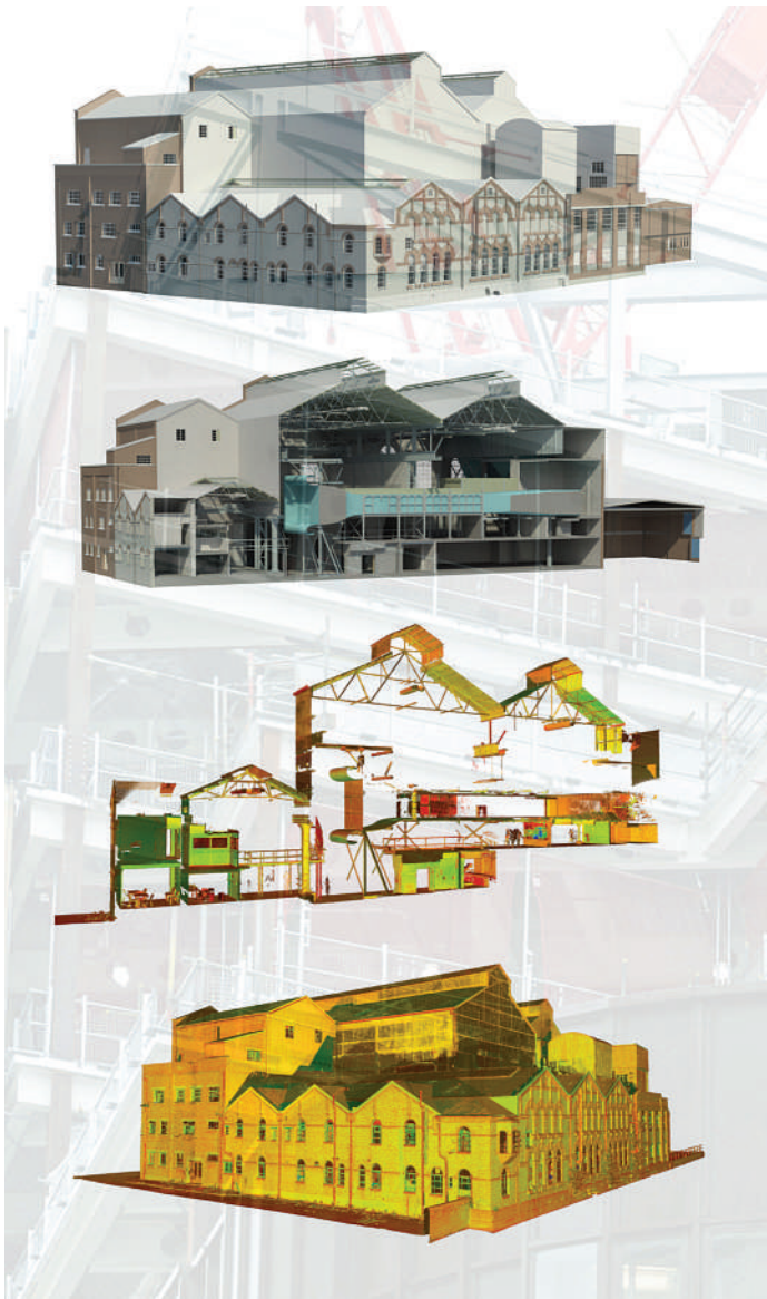
From top: CAD model of an existing “As Built” power station; Elevation Section through CAD model; Section through laser scan point cloud; Complete registered and georeferenced laser scan point cloud
