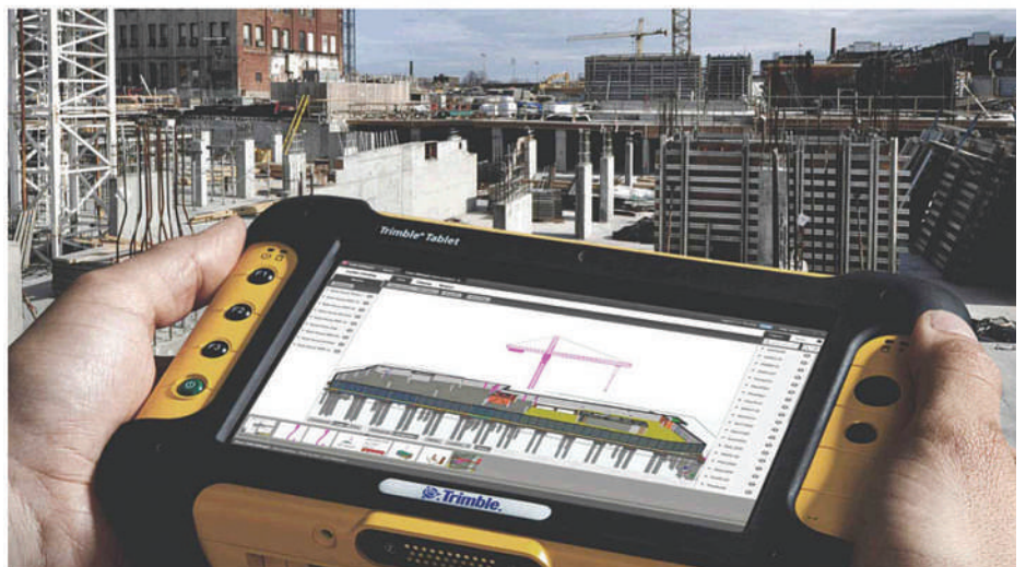
One of the greatest benefits of BIM collaboration software is the opportunity to build a project in a virtual world before construction begins, thus minimising the risk of costly errors and on-site rework, all of which can compromise completion dates and budgets. Tekla Structures Models courtesy of Trimble Solutions UK
