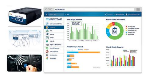
With advanced plug-and-play telematics solutions such as those provided by Geotab, vehicles send data from a multitude of sources, including the engine, the drivetrain, the instrument cluster and other subsystems over modem links to the MyGeotab web-based fleet management software. And by using the latest RFID technology and an NFC fob, operators can quickly, easily, and securely review individual driver trips and driving behaviour. Image Geotab Inc.
