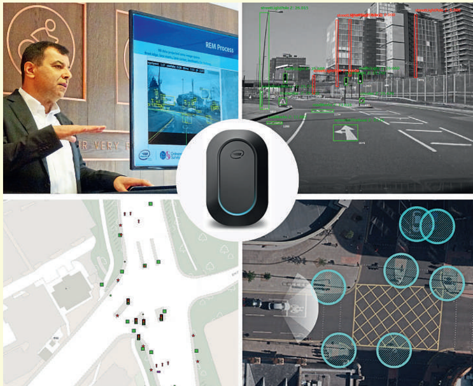
Amnon Shashua (top left) explained how MobilEye’s windscreen-mounted camera (inset centre) is used to detect, capture and classify street-level objects such as lampposts and traffic signals (top right). That data is aggregated and then merged with Ordnance Survey mapping (lower left) to provide real-time information to utility operators, highways authorities and a new generation of driver-assisted and autonomous vehicles (lower right)
