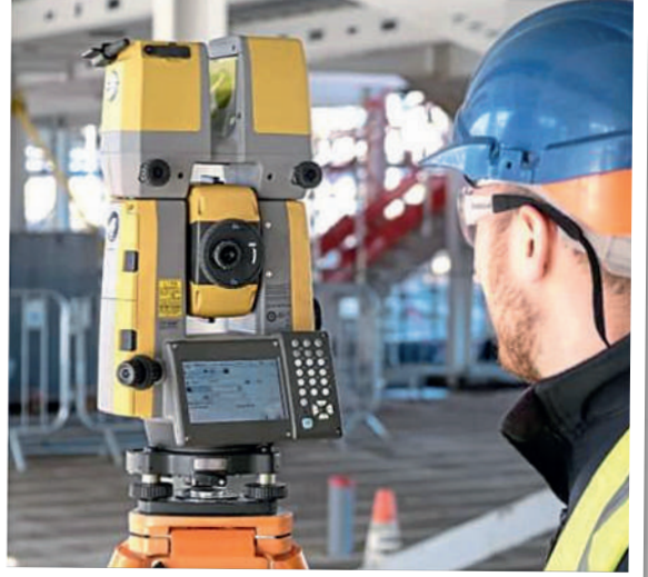
Above left: the Cooper's Hill luxury retirement village under construction (Photo: The Audley Group). Above right: The Topcon GTL-1000 robotic scanning solution being trialled by Balfour Beatty
