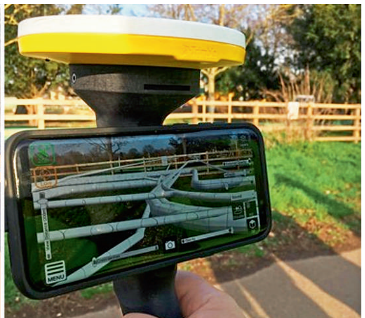
Left: Trimble SiteVision’s small size and easy operation enables professional and non-technical personnel to use in-field, real-time Augmented Reality. Right: Here, it displays a 3D model of underground utilities combined with a live view of existing features.
