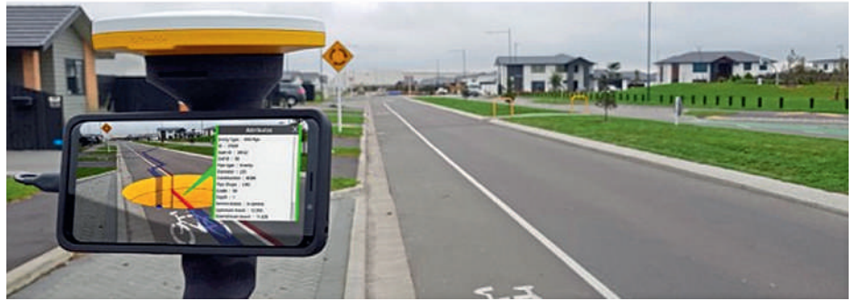
Above: This pedestrian/cycle bridge over the A14 at Swavesey is shown in its on-site location. Trimble SiteVision can use 3D models from CAD and engineering software with live, real-world views. Below: Here, information on buried utilities is combined with real-time on-site visualisation for asset management purposes.
