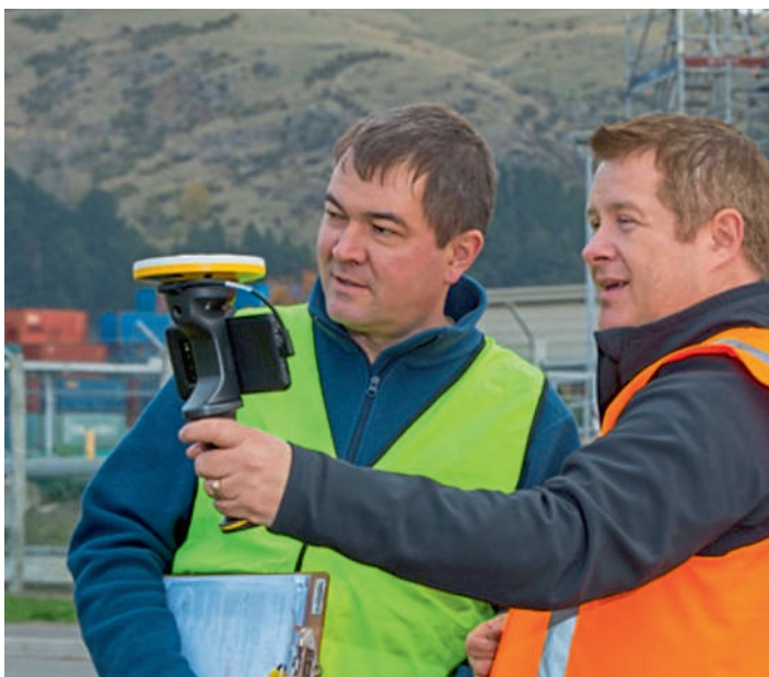
Left: Trimble SiteVision’s small size and easy operation enables professional and non-technical personnel to use in-field, real-time Augmented Reality. Right: Here, it displays a 3D model of underground utilities combined with a live view of existing features.
