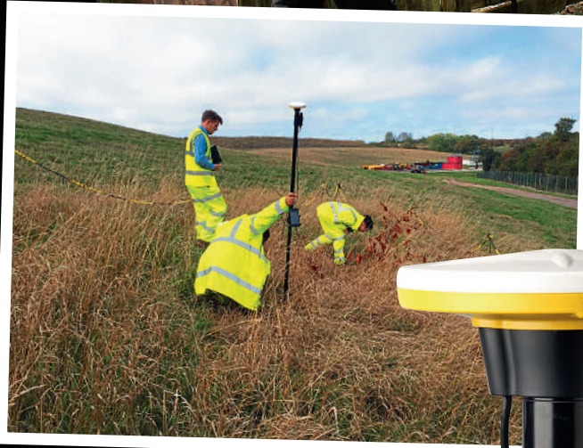
Above: Using Trimble Catalyst and a UAV on a steep embankment infected with knotweed in Swansea
