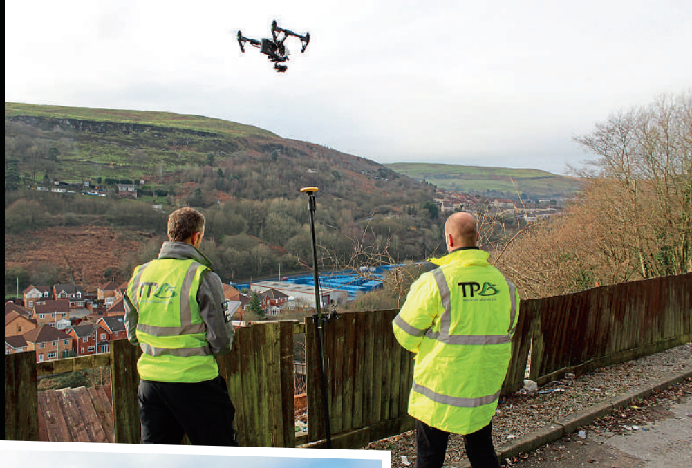
Above: Using Trimble Catalyst and a UAV on a steep embankment infected with knotweed in Swansea
