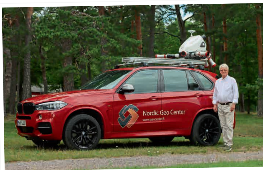
Figure 2. Hannu Heinonen with the survey vehicle equipped with the RIEGL VMX-2HA Mobile Mapping System. Picture: Nordic Geo Center
