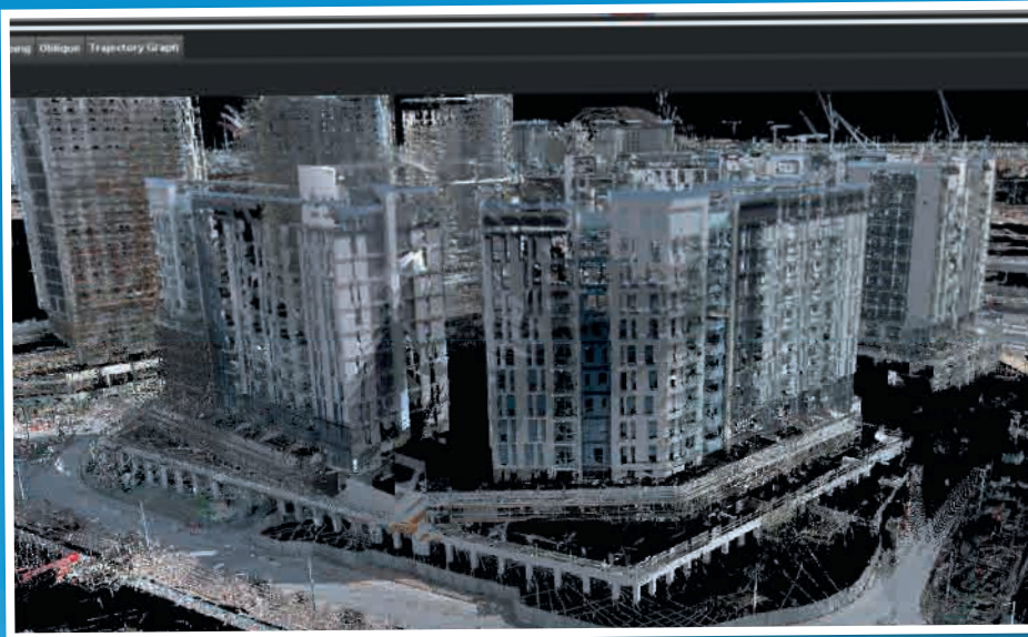
A point cloud view of Dubai's Exhibition Center which will host the world EXPO 2020
