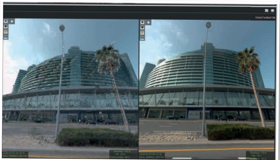
Dubai's Festival City, captured simultaneously by the MX9's laser scanners and cameras. The MX9 acquired 360° panorama images every five seconds and two million 3D points per second.
