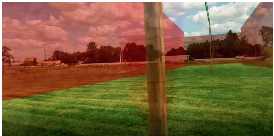
A pole and line design seen in AR includes visualisation of right-of-way as transparent red walls
