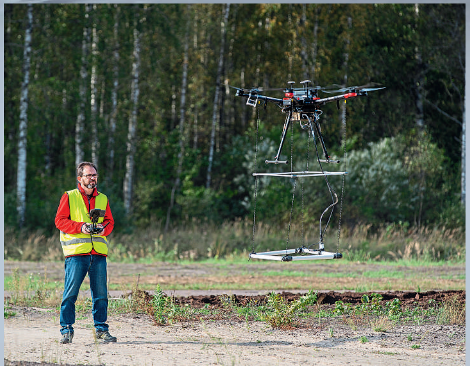
Alexey Dobrovolskiy conducts first tests of a metal detector after sensor integration with a UAV © SPH Engineering
