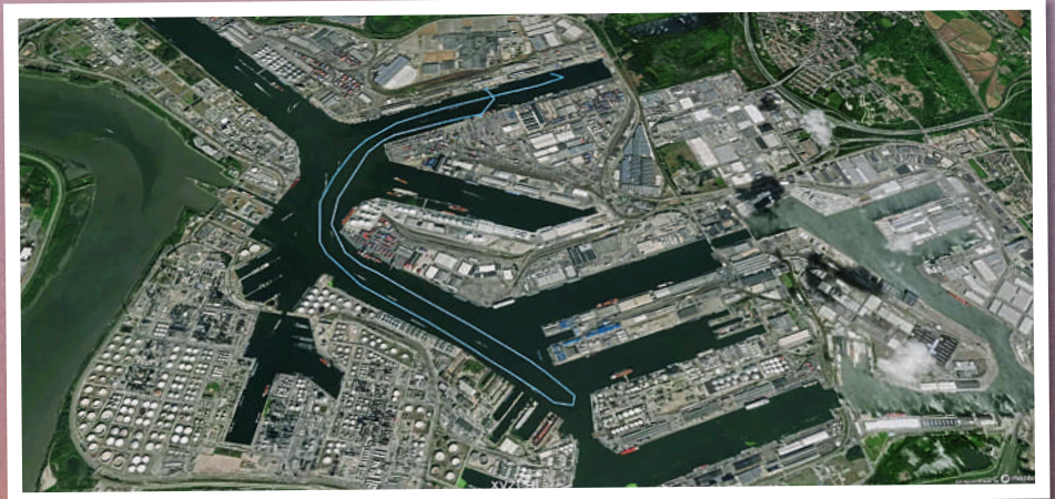
Figure 2. A likely illegal degassing event by a tanker moving outside and back inside a dock following a "sight-seeing" trip to get rid of the remaining vapours. Algorithms developed by xyzt.ai with Port of Antwerp
