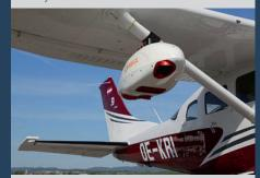
The EASA (STC) approved RIEGL VQX-1 Wing Pod now provides a fully integrated, modular airborne laser scanning system for user-friendly operation with single-engine Cessna 172, 182 and 206 aircraft.
