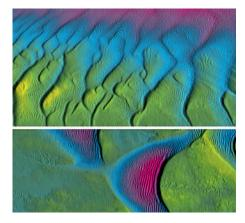
Examples from AI trials conducted in the North Sea off Lowestoft by specialists from the University of East Anglia and GeoAcoustics. Top: a section of a 780m X 380m grid of the Stanford Channel acquired with GS4 showing sand waves between 0.08m and 4m in height. Lower: Sample from a calibration area 190m x 550m east of Holm Sand (50cm resolution)
