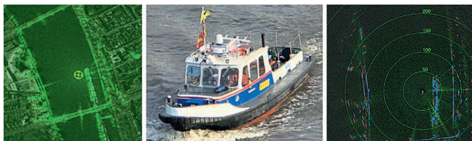
Navtech's radar-based localisation solution, Terran360, being successfully trialled with BAE Systems on London's River Thames to test performance and usability. Above left: Raw radar data collected on the test vessel and overlaid on a satellite image of the same location. Above centre: Terran360 radar mounted on BAE Systems' survey vessel. Above right: Radar point clouds (shown by blue and red dots) extracted by Terran360 to localise vessel position within the environment
