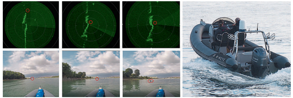
Results from Navtech 2022 field trials of W-band radar on the River Torridge in Devon. Above left: Radar data (top) to detect kayaker (circled in red) from a range of around 250 m. The images immediately below were taken simultaneously by a GoPro camera aboard the trials vessel. Right: The vessel used for field trials data collection, fitted with a Navtech Terran360 radar
