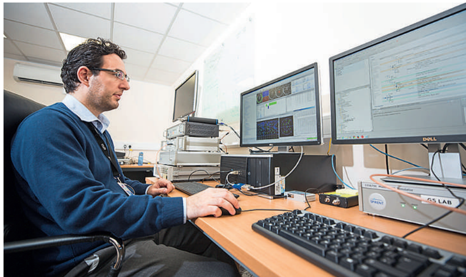
The UK is possessed of a good range of PNT test facilities, such as this multi-constellation GNSS test rig from Spirent Communications based in Paignton, Devon.
