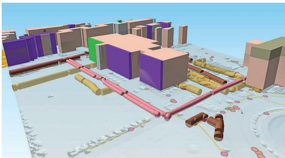
Ground Penetrating Radar identifies subsurface utilities beneath a 3D model of buildings classed by energy efficiency
